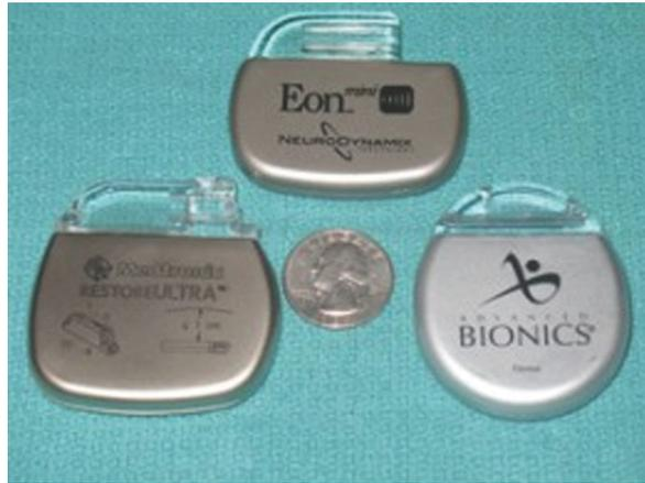
Fig 4. Implantable batteries in rechargeable and non-rechargeable varieties.
